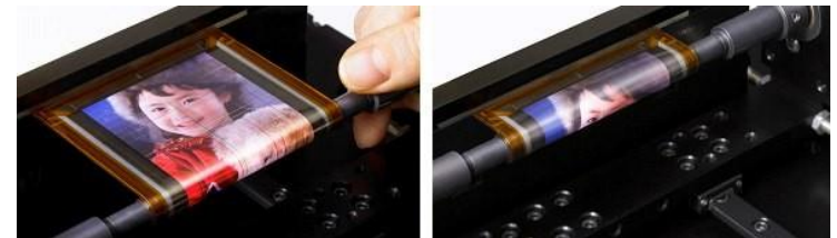
Demonstration of a 4.1" prototype flexible display from Sony
