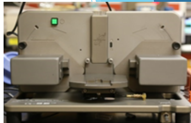
Woollam Ellipsometer: thin film thickness and refractive index measurements
