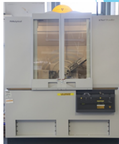
PANalytical PXRD: For powder crystallographic analysis. Temp. measurements in the -173 - 400^{\circ}\text{C} range
