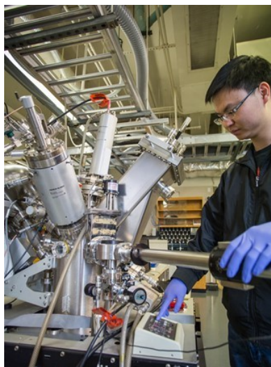
XPS: For surface elements survey and depth profiles
